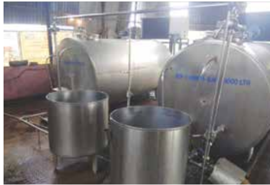
Picture 2.4: Bulk Milk Coolers (BMCs) in a village in Andhra Pradesh
