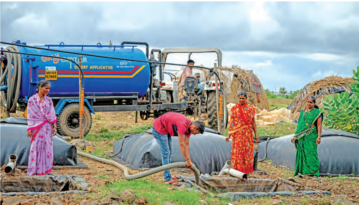
Slurry lifting using a slurry applicator
